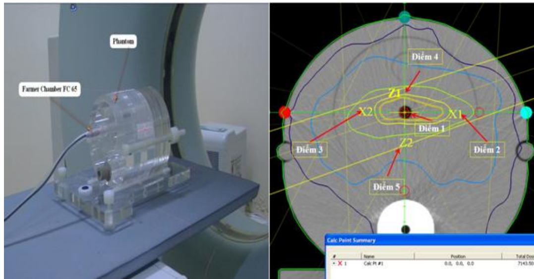
The dose distribution on cylindrical phantom at isocenter of case.
